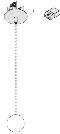
Plasterboards Ceiling rose with driver 1 lamp
